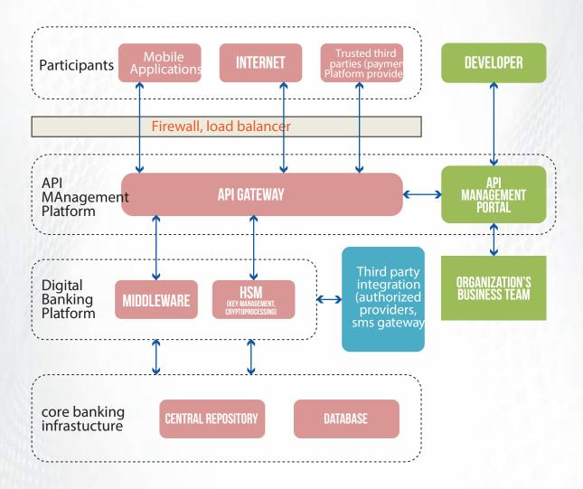
The above shows the flow of data from originating channels (Mobile apps, TTPs) toward the core banking infrastructure. This end user could be a bank customer or a trusted third party utilizing the services provided by the bank via APIs.
